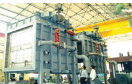
2590x2590 mm Diverter Flap Valves for GE Exhaust System of LM 6000 Gas Turbine through BSES
