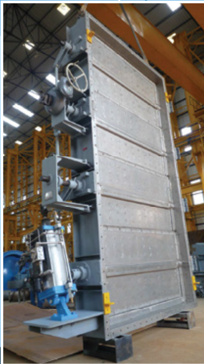
Louvre Damper for FGD Application
