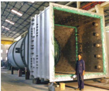
Silence & Stack for GE M S 6001 Turbine supplied to Inso/Nuovo Pignone for Reliance Petroleum, India
