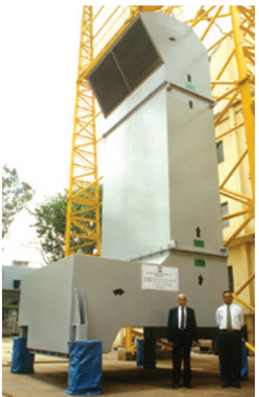
VBV Silencer to GE Packaged Power Systems, Houston, USA for GE LM 6000 Gas Turbine
