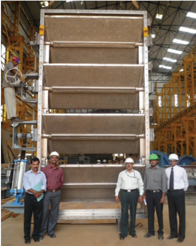
Multiflex ( Multi Louvre) Damper with Hastalloy-C Liner – FGD plant at JSW , Ratnagiri
