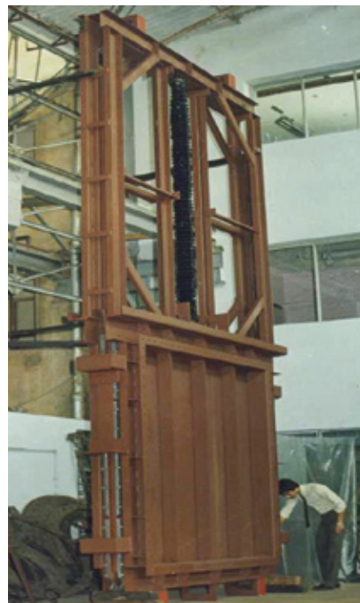
3000mmx 3000mm Glandular Guillotine Isolator supplied to Ansaldo, Italy
