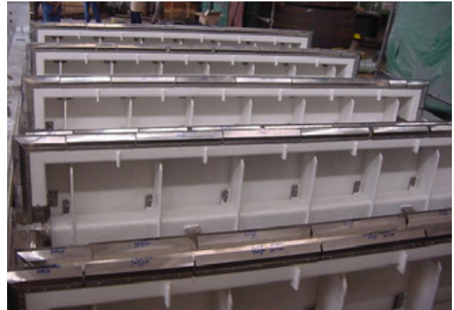
Duplex Louvre Damper with Poly Glass Lining – Reliance Dahanu FGD Plant
