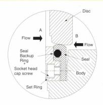
Fouress #300 rating high performance butterfly valves are reliable, well proven design provides bi-directional shut-off.
